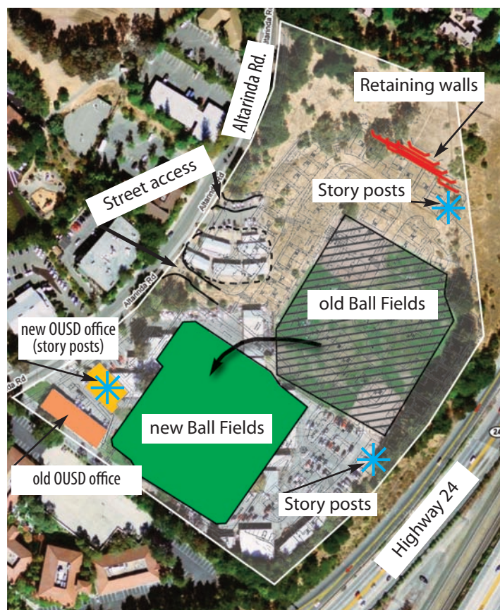
The map above illustrates the site; the old and new location of the ball park, OUSD office, new retaining walls and also the position of the new access roads Graphic Andy Scheck
