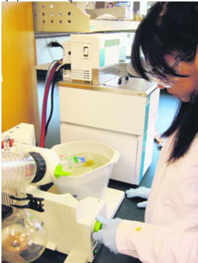
Elizabeth Sandoval-Torres uses a rotary evaporator to remove solvent and isolate her reaction product Photo Valerie Burke
