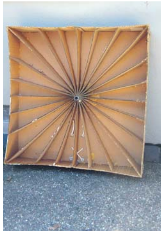
The frame of the solar stovetop is made of cardboard Photo Sophie Braccini
