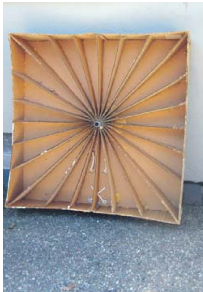
The frame of the solar stovetop is made of cardboard
