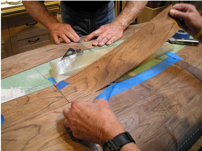
Gluing strips in place
