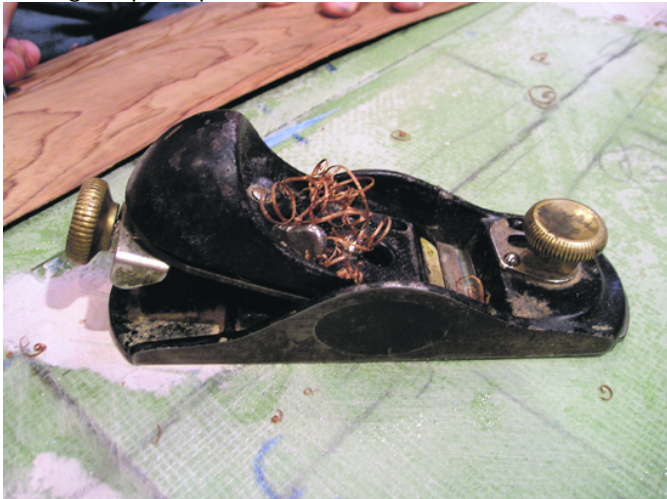
Hand planer on canoe bottom, showing fiberglass layer
