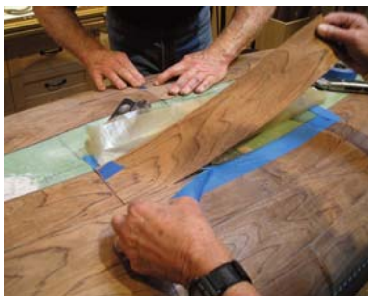
Gluing strips in place
