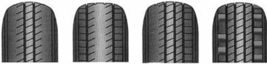
UNDER-INFLATION OVER-INFLATION POOR ALIGNMENT UNEVEN WEAR
