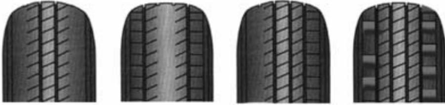
UNDER-INFLATION OVER-INFLATION POOR ALIGNMENT UNEVEN WEAR
