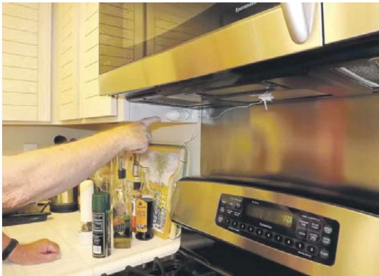
A heat sensor mounted above the oven can alert Justin Pickering if his father has left the burner on.
