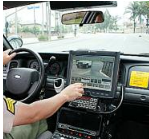
An officer uses a license plate recognition system (ALPR) inside his patrol car. Photo public domain
