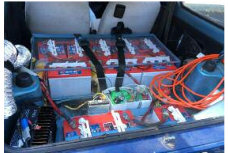
The view of the back of Thelen's 1976 Honda Civic with 11 of its 15 batteries
