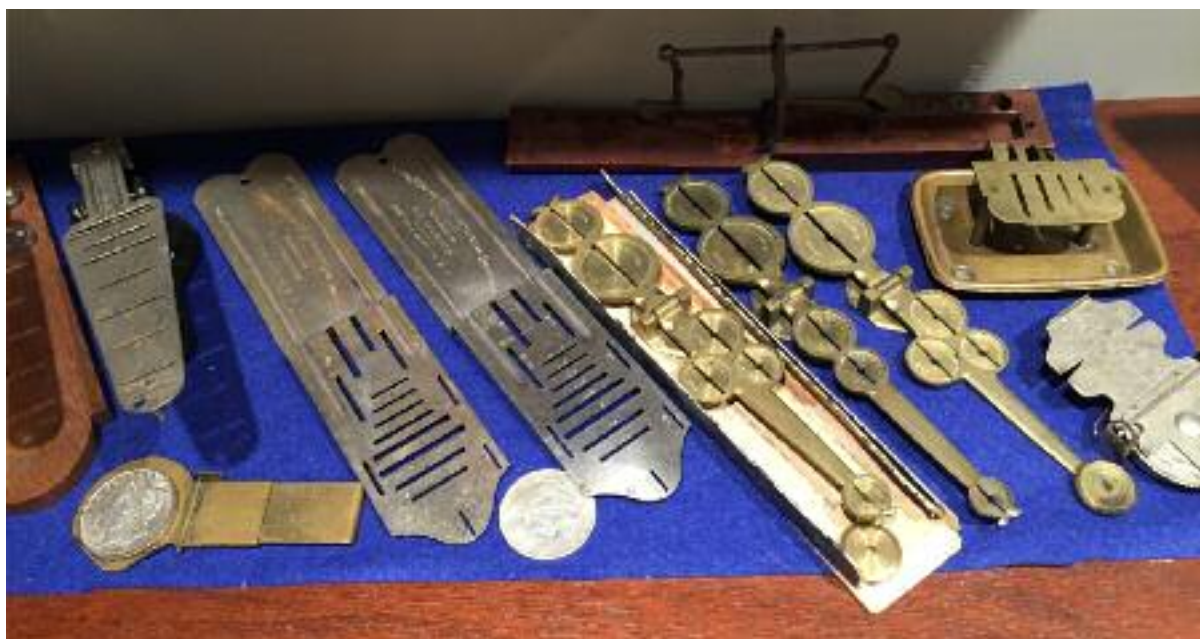
A collection of counterfeit coin detectors from Doug Scougale's collection. The slots verified proper coin size, the scale showed whether the metal was truly precious metal or a counterfeit filled with lead. Photo Cathy Dausman
