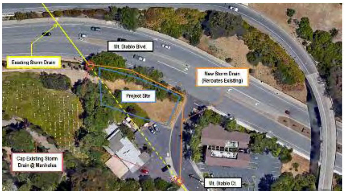
Image provided by EBMUD depicting location of existing and future storm drains.
