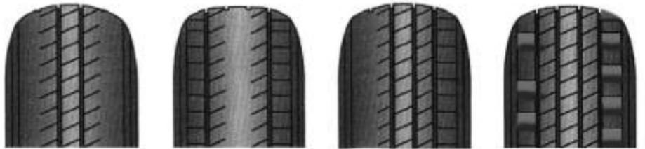
UNDER-INFLATION OVER-INFLATION POOR ALIGNMENT UNEVEN WEAR
