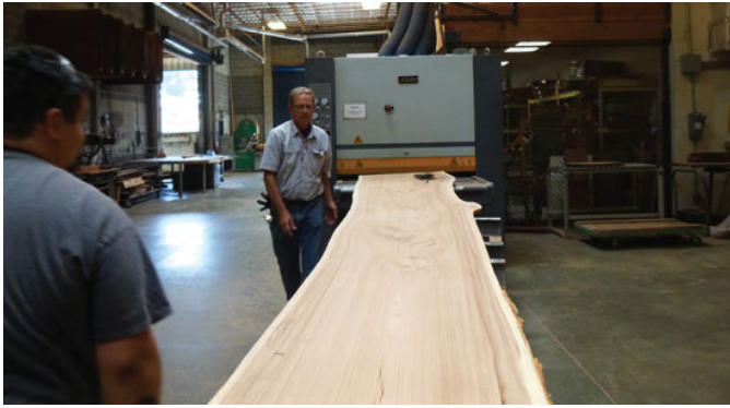
This single piece oak board that will eventually become a bar gets set to go through the sander. Photo Sophie Braccini
