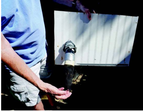
Mesh attached to a pipe and reduced to a half-inch at the end was used to trap bees out of Munson's home. Photos Cathy Dausman
