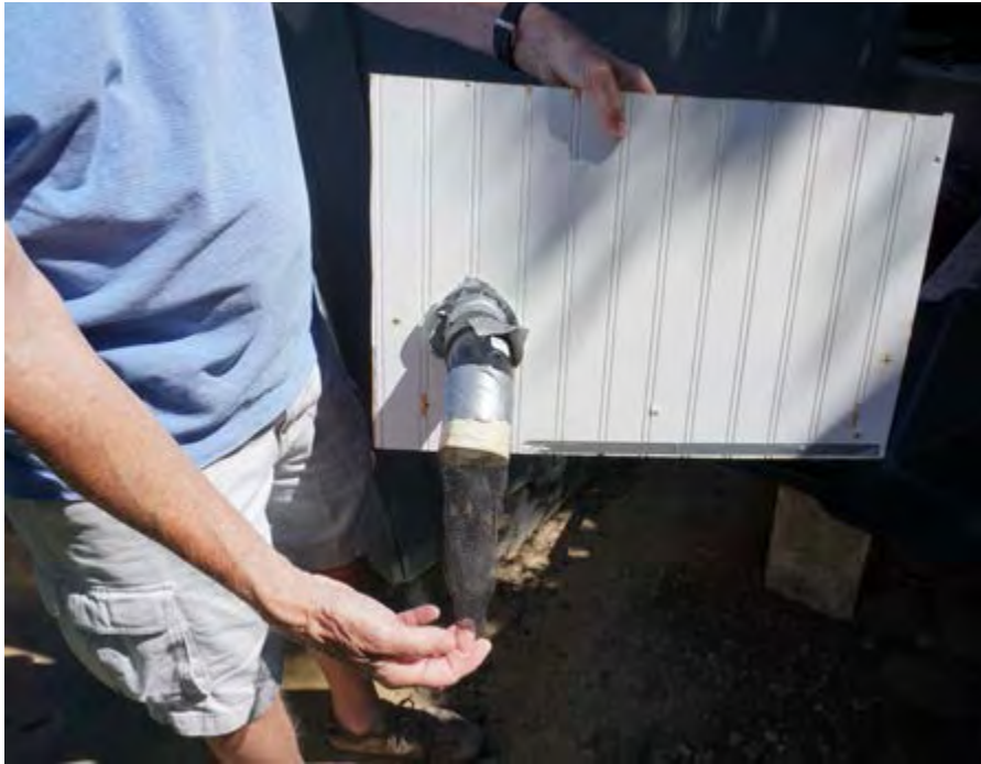
Mesh attached to a pipe and reduced to a half-inch at the end was used to trap bees out of Munson's home.
