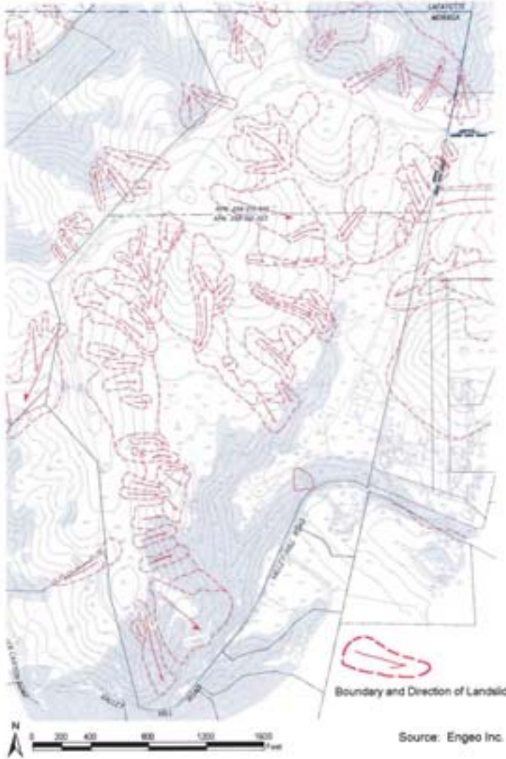
Map of existing landslides – a concern identified in the Bollinger Valley Project Environmental Impact Report.
